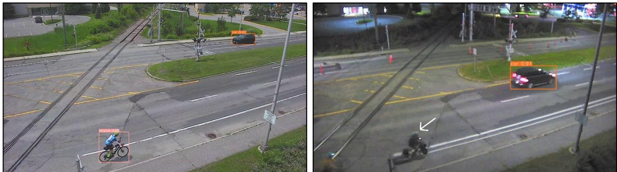
Figure 15: Example detection on day time image (left) and night-time image (right) captured by the PTZ_ingress camera. The cyclist on the left image captured during the day was accurately detected by the model, while another cyclist in the same position (denoted by the white arrow) captured by the same camera during the night was missed.
