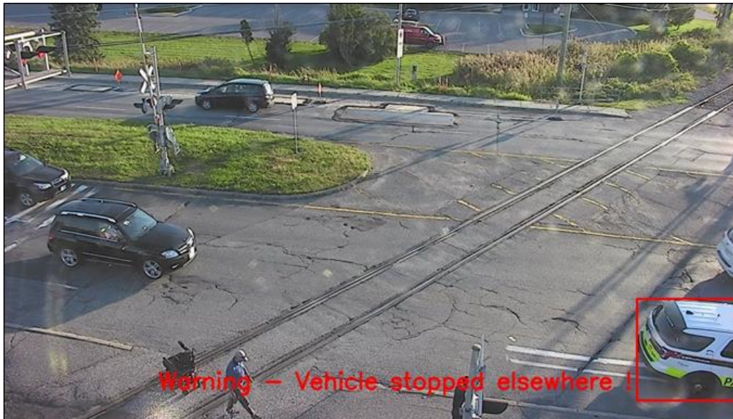
Figure 28: Vehicle (with a red rectangle) detected by the algorithm as stopped elsewhere.
