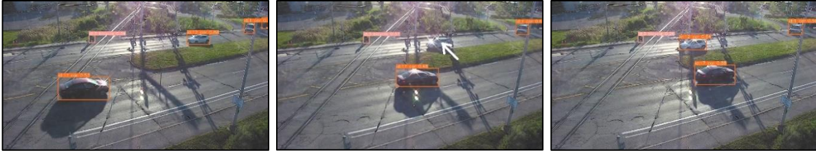
Figure 22: Example of detections on PTZ_ingress camera images under strong glare conditions; (left image) the white car on the top-right corner of the image travelling along the far lane was accurately detected before entering the glare zone; (middle image) the car was missed in the next frame sequence as it passed through the strong glare zone (denoted by the white arrow); (right image) the car was detected again as it left past the glare zone. (Best viewed when zoomed in.)
