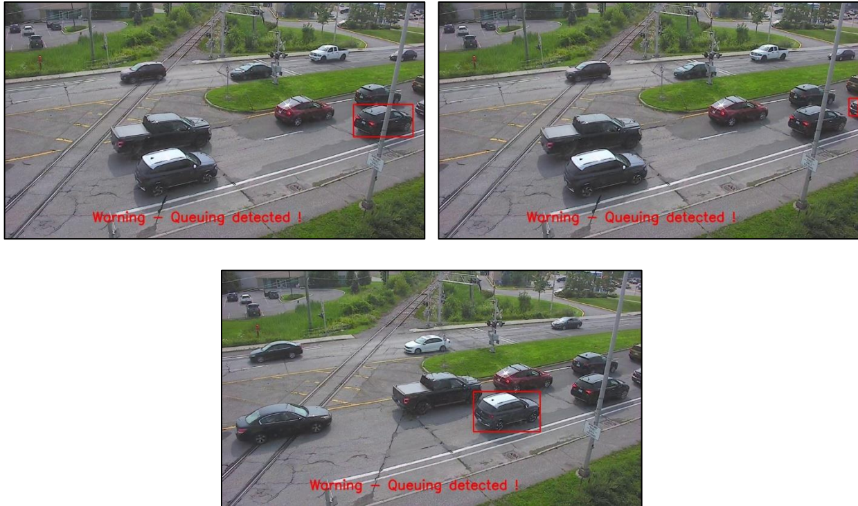
Figure 30: Queuing event involving three vehicles (each with a red rectangle) detected by the algorithm in lane 4.
