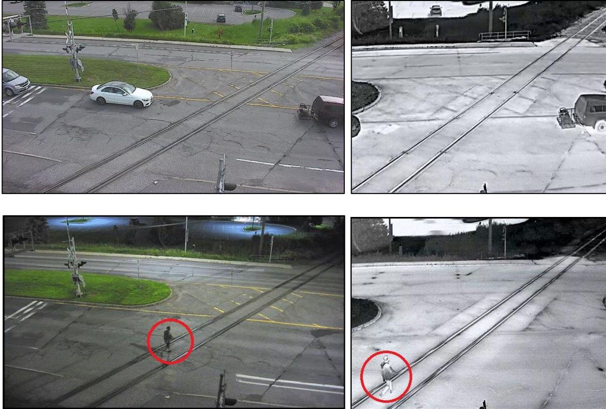
Figure 6: Examples of some of the potentially unsafe events captured by both PTZ and thermal cameras. The top row depicts a scenario where cars queue up on the egress of the crossing, extending past the crossing into the ingress area. The bottom row shows a pedestrian (encircled in red) intruding into the railway right of way.
