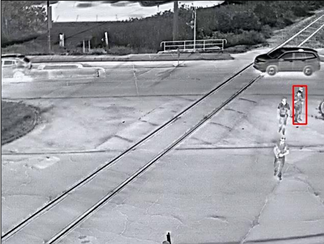
Figure 31: Two pedestrians (with the red rectangle), walking side by side, were detected as one person.
