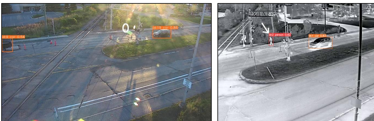
Figure 23: Lens flare causing the pedestrian (encircled in white on the left image) to become completely obscured in the PTZ_ingress camera image. The corresponding thermal image (right) allowed the model to detect the pedestrian accurately.
