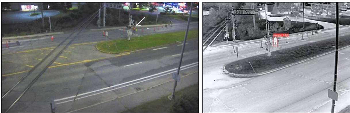
Figure 17: VRU detection during night time on PTZ (left) and thermal (right) camera images. While the model trained on PTZ camera images failed to detect the VRU (denoted by the white arrow on the right image), the model trained on thermal camera images was able to detect it in the corresponding thermal camera image.
