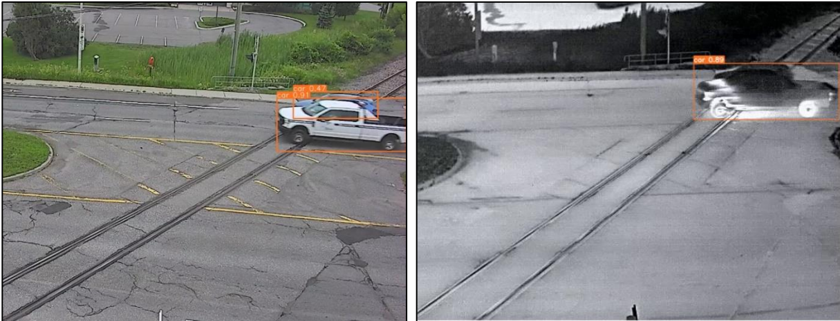
Figure 19: Two occluded cars captured by the PTZ_egress (left image) and Thermal_egress (right image) cameras. The model trained on the PTZ camera images was successful in detecting both cars (one in the foreground and a second in the background) as shown in the left image, while the model trained on the thermal camera images failed to detect the occluded car as revealed in the right image.
