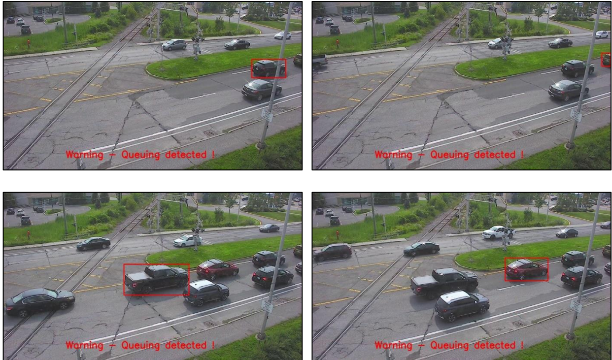
Figure 29: Queuing event involving four vehicles (each with a red rectangle) detected by the algorithm on lane 3.
