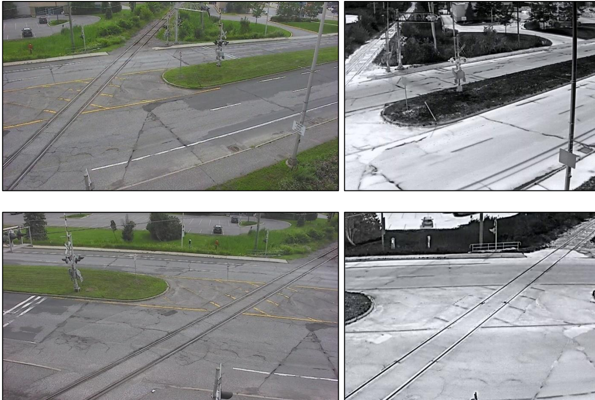
Figure 2: Ingress view of the crossing captured by RGB camera (top-left) and thermal camera (top-right); egress view of the crossing captured by RGB camera (bottom-left) and thermal camera (bottom-right). Northbound road traffic is in the far lanes and moves from right to left, and southbound road traffic is in the near lanes and moves from left to right.
